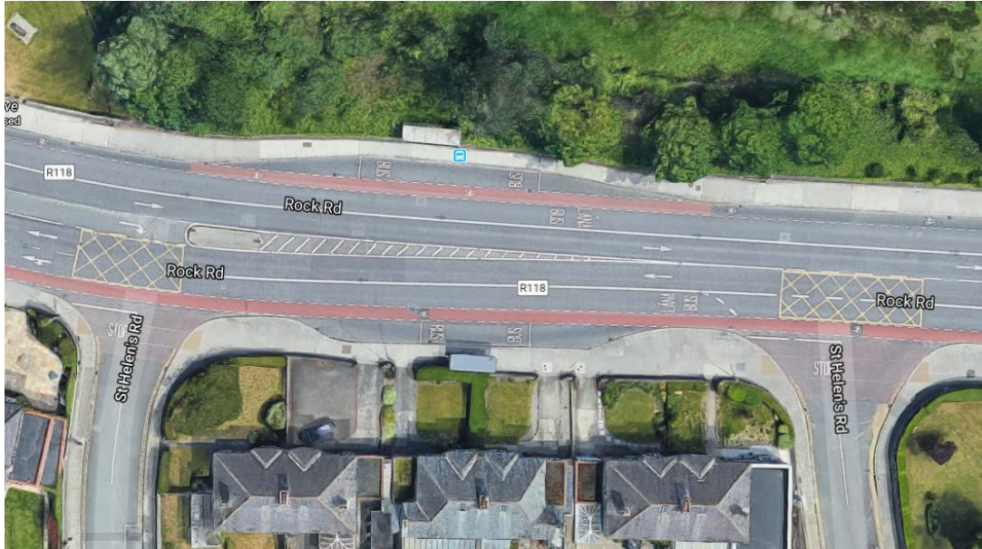
Figure 19: Pedestrian Crossings - No Pedestrian Crossing at either end of St Helen's Road
